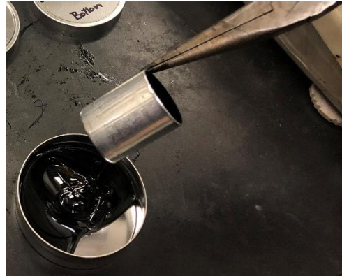
Figure 3. Binders Taken Out from the Various Cigar Tube's (top, middle, and bottom) Portions
