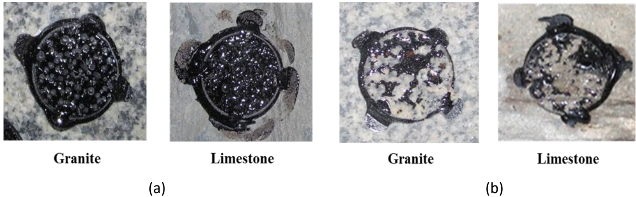
Figure 5. BBS Test Failure Type; (a) Mainly Cohesive Failure, (b) Mainly Adhesive Failure (Moraes et al., 2011)
